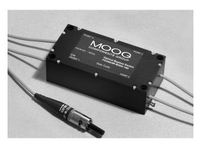
The multimode 2x2 moving-mirror optical bypass switch meets all the requirements of the FDDI Physical Medium Dependent (PMD) standard and SAFENET specifications for fiber optic data network applications. The highly reliable performance of the device is made possible by its unique silicon micromachine based switch design. A sealed, ruggedized housing isolates the optical components from external shock and vibration effects.
